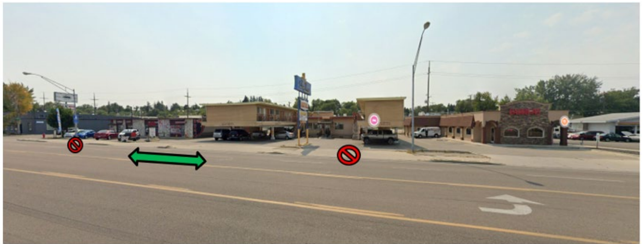
Figure 2: ITD's Access Management Plan. Limit access to allow only one approach per parcel. Green arrow represents ITD's requirements to limit the approach to 40ft.
