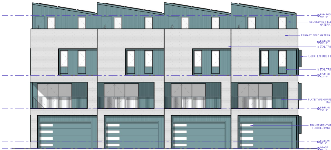
1 BUILDING 6 - WEST ELEVATION SCALE: # 3/16" = 1'-0"
