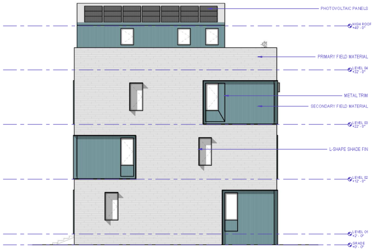
2 BUILDING B - SOUTH ELEVATION (ALWORTH) SCALE # 3/16" = 1'-0"
