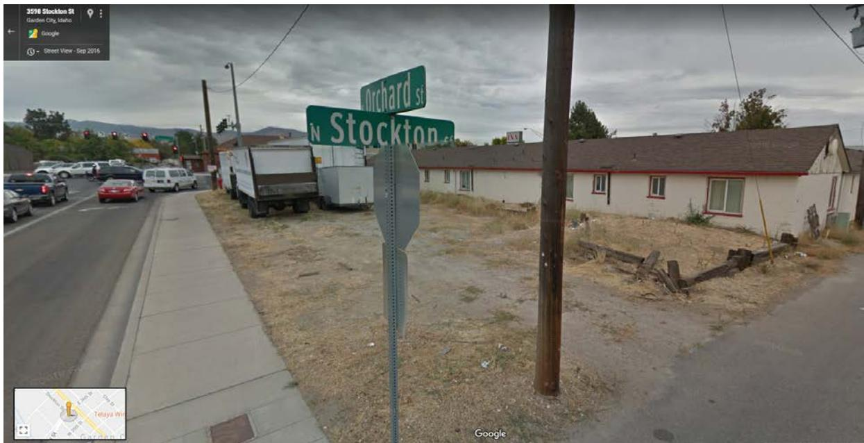
The proximity of this infrastructure to the proposed entrance may present a significant impact to the health, safety, and welfare of the community. There appears to be a significant risk of a vehicle or trailer hitting the power pole or guide wire, which could interrupt power service in the area.
